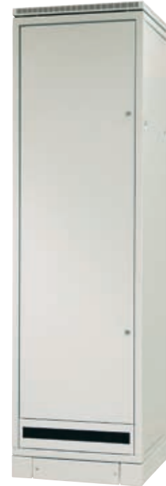
[7] Solid steel, shortened door with single-point locks + 1 piece of 3 U module panel with brush strip, mounted under the shortened door
