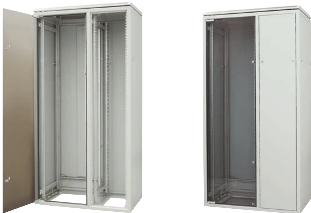
SZB cabinet 1000 mm wide, double-sectioned. Left section equipped with 19" mounting profiles. Right section with mounting angles in 300 mm spacing.
