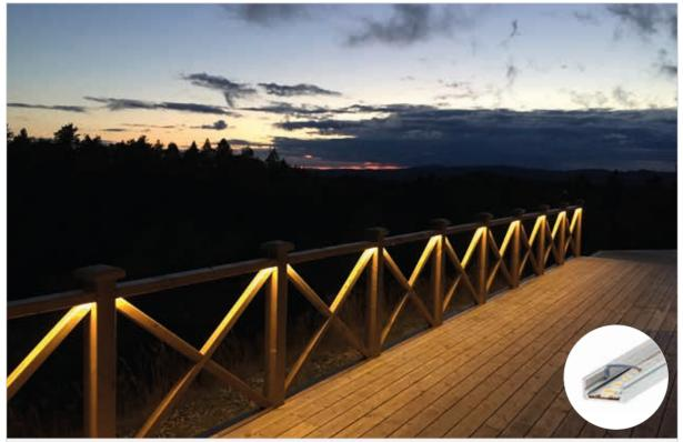
Profile: A1 Standard // LED-strips: 4,8W/m IP67
