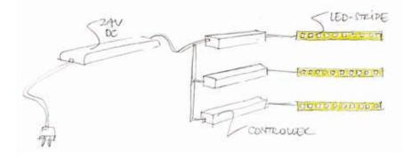
If the installation requires more than 10A, repeaters should be chosen to expand the capacity. A repeater will act as a slave module for the controller and perform the same tasks with 100% accuracy. The master controller should only control repeaters which are connected to the LED strips.
