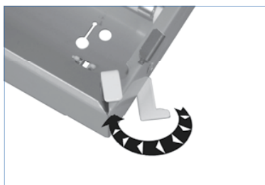
PRINCIPLE OF FIXING THE COVER
