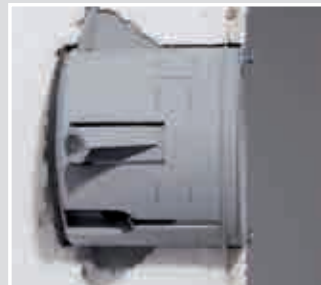
The lip at the back forms a sealing barrier to the insulation material and prevents air draughts along the box.
