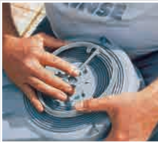
Clip the front ring onto the housing.
