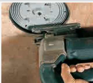
Open front part using a fretsaw.
