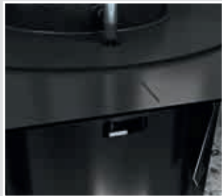
Align plate screws of the sealing cylinder with the markings and tighten.
