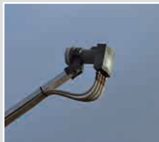
4 coaxial cables are connected here for reception.
