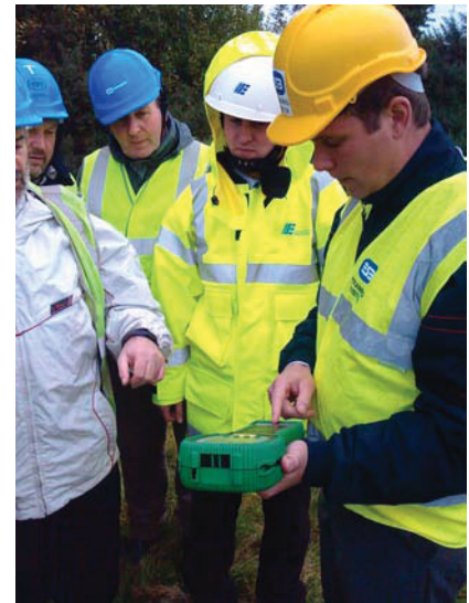
Measuring of earthing resistance.
