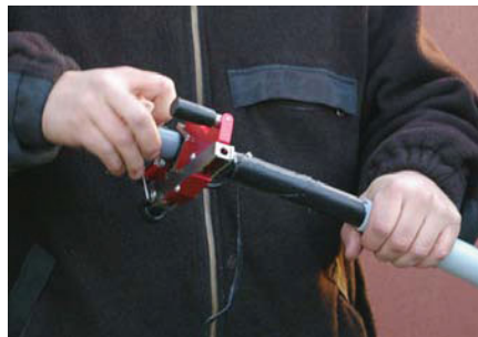
FBS1722, for stripping of outer conductive layer gives a very smooth result.
