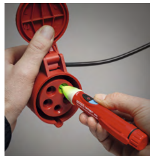
Phase sequence testing green = clockwise
