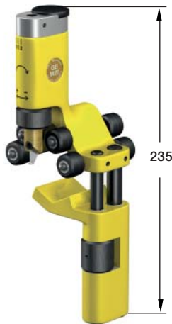
GB-M20 Cutting tool for cable sheath and XLPE-insulation: Diameter: Ø 15-50 mm Cutting depth: ≤ 8 mm
