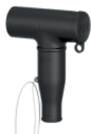
IH-A 24630, IH-A 42630 Insulating sealing hood of flexible rubber with outer conductive layer and an already installed insulating hood. To be installed in HDC-A 630 instead of cable connector in order to temporarily insulate 630 A switchgear or transformer bushings.
