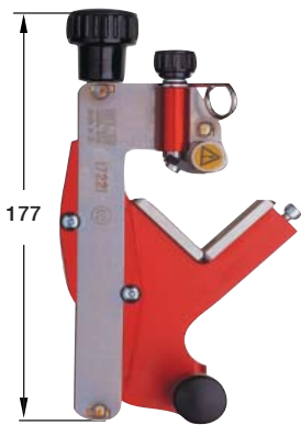
Intercable No. FBS 1722 1 Stripping tool for the vulcanized, outer conducting layer of XLPE-insulated cable Ø 10-52 mm. The tool is supplied in a rigid case with a tube of silicone grease.
