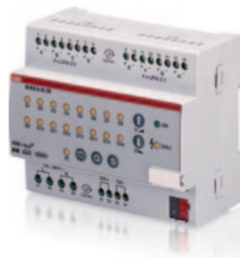
Control via 16 lighting groups. Up to 8 lighting groups can be controlled with 8 light sensors. Master-slave, staircase light and Scene mode round off the functions.
