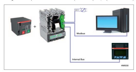
Positioned in the right-hand slot of the circuit-breaker, the Ekip Com accessory connects to the Ekip LSI, Ekip LSIG, Ekip E-LSIG or Ekip M-LRIU trip unit via connector supplied with Ekip Com and to the MOE-E via connector be present on MOE-E behind. Six cables come out of Ekip Com of which two are required for auxiliary supply, two for connection to the Modbus and two for connection to Internal Bus.
