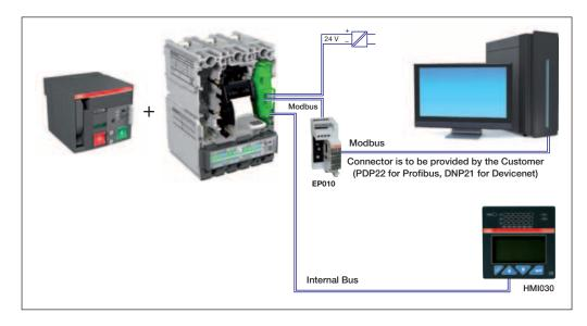
Positioned in the right-hand slot of the circuit-breaker, the Ekip Com accessory connects to the Ekip LSI, Ekip LSIG, Ekip E-LSIG or Ekip M-LRIU trip unit via connector supplied and to the MOE-E via connector be present on MOE-E behind (MOE-E connection is optional for this configuration). Six cables come out of Ekip Com, of which two are required for auxiliary supply, two for connection to the EP010 and two for connection to Internal Bus.
