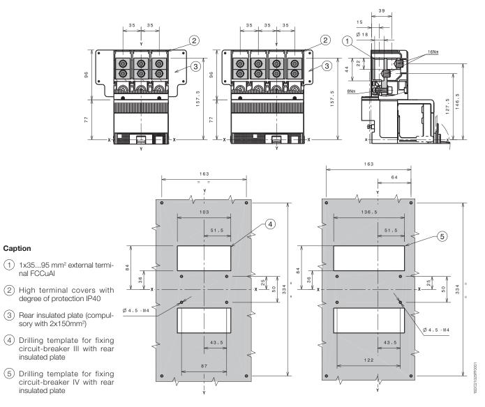
Tmax XT3 - Terminals for plug-in circuit-breaker
