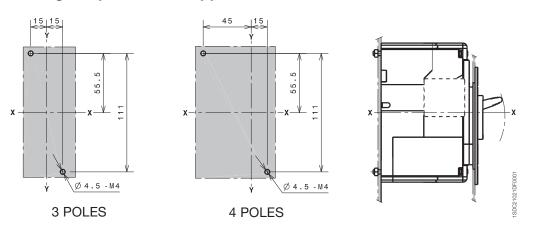
Tmax XT2 - Installation for fixed circuit-breaker
