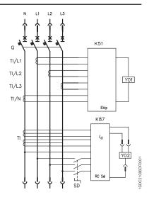
Four-pole circuit-breaker with electronic trip unit and RC Sel residual current release
