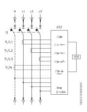
Three-pole or four-pole XT4 circuit-breaker with Ekip E-LSIG microprocessor based release
