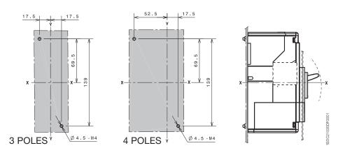
Tmax XT4 - Installation for fixed circuit-breaker
