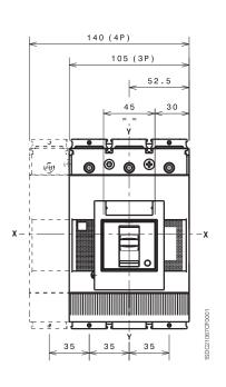
Tmax XT3 - Terminals for plug-in circuit-breaker
