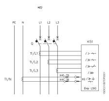
Three-pole fixed version circuit-breaker with current transformer on the neutral conductor outside the circuit-breaker
