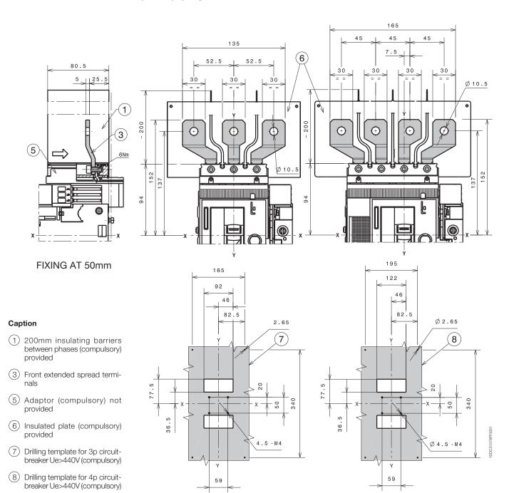
Tmax XT2 - Terminals for withdrawable circuit-breaker
