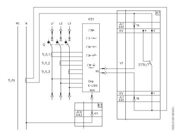
Advisable diagram for plug-in or withdrawable version three-pole circuit-breakers with current transformer and voltage connection on neutral conductor, external to circuit-breaker
