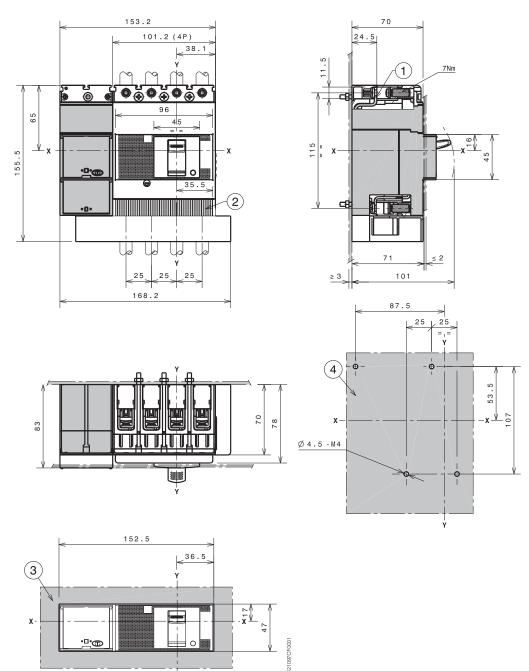
Tmax XT1 - Installation for plug-in circuit-breaker
