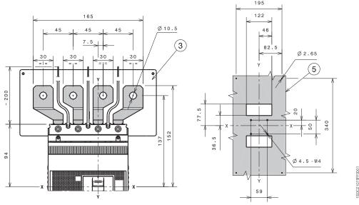
Tmax XT2 - Terminals for plug-in circuit-breaker
