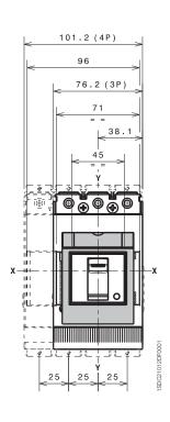
Tmax XT1 - Terminals for plug-in circuit-breaker
