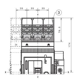
Tmax XT4 - Terminals for withdrawable circuit-breaker
