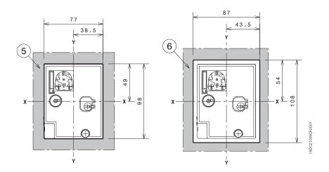
Tmax XT2 - Installation for fixed circuit-breaker
