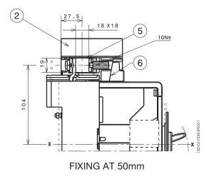
Tmax XT4 - Terminals for plug-in circuit-breaker
