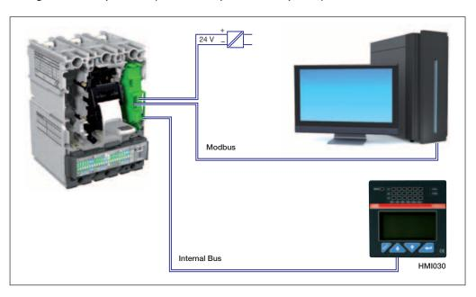
Positioned in the right-hand slot of the circuit-breaker, the Ekip Com accessory connects to the Ekip LSI, Ekip LSIG, Ekip E-LSIG or Ekip M-LRIU trip unit via connector supplied. Six cables come out of Ekip Com, of which two are required for auxiliary supply, two for connection to the Modbus and two for connection to Internal Bus.
