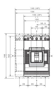
Tmax XT4 - Terminals for withdrawable circuit-breaker
