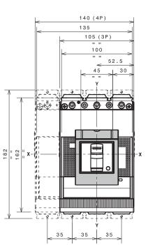
Tmax XT4 - Terminals for plug-in circuit-breaker
