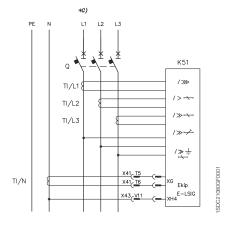
Fixed version three-pole XT4 circuit-breaker with Ekip E-LSIG with current transformer on neutral conductor, external to circuit-breaker
