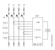
Four-pole circuit-breaker with Ekip N-LS/I electronic trip unit
