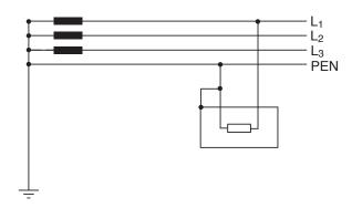
3. TN-C-S: the neutral and protection functions are partly combined in a single conductor called PEN and partly separate PE+N
