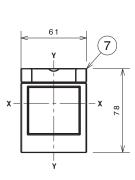
Tmax XT1 - Installation for fixed circuit-breaker
