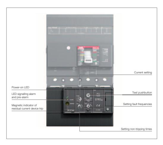
The RC B Type residual current release, to be used in conjunction with the XT3 circuit-breaker, has the following features:
