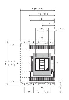
Tmax XT2 - Terminals for withdrawable circuit-breaker
