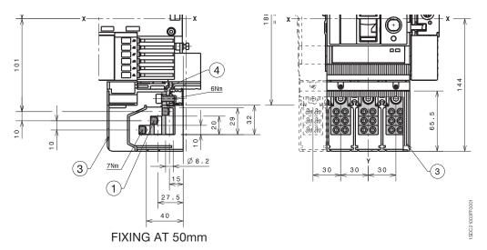
Tmax XT2 - Terminals for withdrawable circuit-breaker
